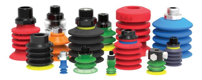
This family is designed for height differences, slightly curved planes and uneven surfaces. Applications such as bag handling, cardboard, high temperature or if the need is specifically to touch a food item as they are also available in material that complies with the FDA (FDA 21 CFR 177.2600) and meets EU's regulation EU 1935/2004.
