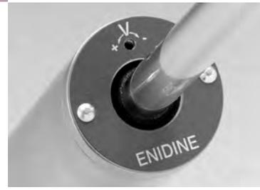
Turn adjustment pin 1 3/4 turns open to provide minimum damping force. Turn adjustment pin fully closed to provide maximum damping force.
